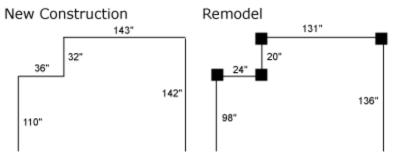
IMPORTANT: Measurements should be to the outside corner for new installations and to the post or column for remodels.
